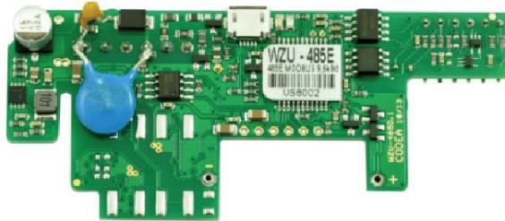
The processor unit uses both modules to communicate over ModBus® or BACnet™.
