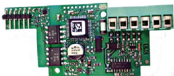
In addition to the M-bus connection facility, the WZU-MI module has 2 pulse inputs to connect metering pulses from hot and cold water meters with Reed contact, relay or open collector. The cumulated volume is calculated based on the pulses and the set pulse valency, stored in the processor unit at 5-minute intervals and passed on via M-bus.
