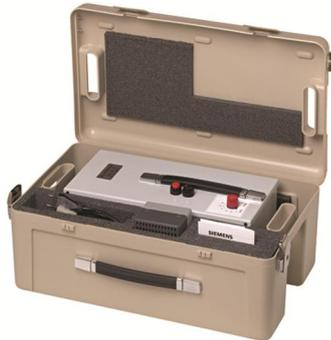
The test lamp LE3 is used to test the function of all flame detectors over distances up to 10 m. It is housed in a transportable case together with the required accessories. In addition, the case enables the test lamp to be kept in a dust-free condition.
