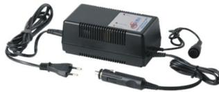
Charger as spare part for charging the batteries RE7T-B
