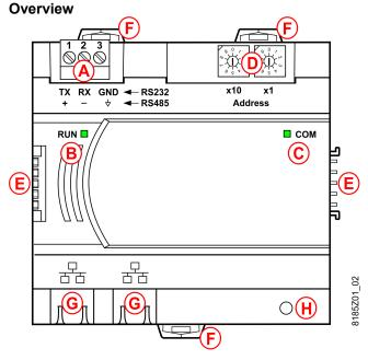
A Plug-in screw terminal for RS232 and RS485 (Changeover via software)
