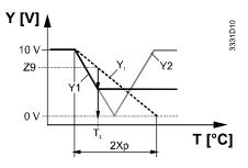
1-stage heating and 1-stage cooling Minimum limitation, acting on Y1 and Y2
