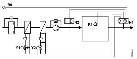
Extract air temperature control through control of the heating and cooling valve in sequence, with outside temperature compensation, remote setpoint adjuster, and limitation of the supply air temperature
