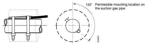
Sensor can be mounted on a piece of pipe with no lagging or underneath the lagging.
