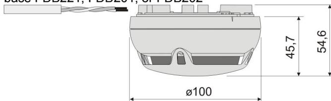
with base FDB222 for flush mounting, only for recess-mounted cable entry
