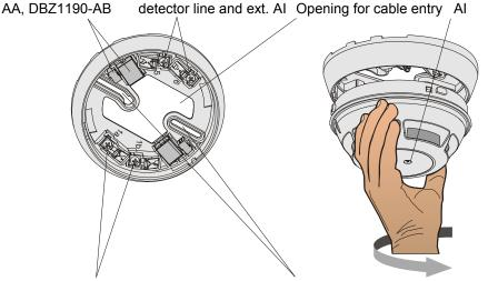
Connecting terminals detector Mounting slots min. 40 mm up to max. 90 mm line and ext. Al
